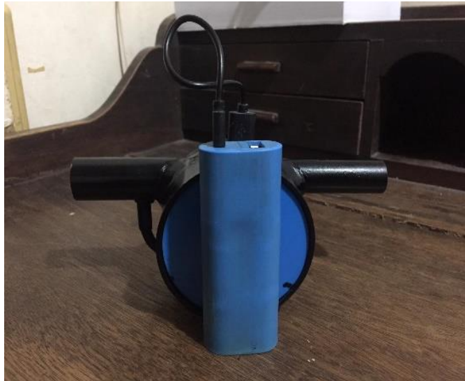
Fig. 3. The Micro-Hydro Generator Turbine.
